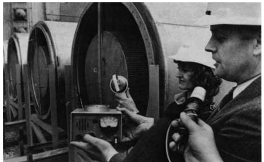
Radiation protection technician Beverly Della Loggia and Robert C. Arnold show the media a method of checking for airborne radioactivity. This check was made March 10 this year before the first time since the accident that humans entered the airlock leading to the Unit 2 Reactor Building. The contents of the airlock were cleared into the atmosphere through the vents next to Della Loggia and Arnold. The two made the test while the airlock was being cleared for the entry on March 13.
